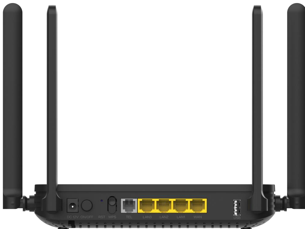
Figura 2: A XSI-G410-W6 vista de trás
